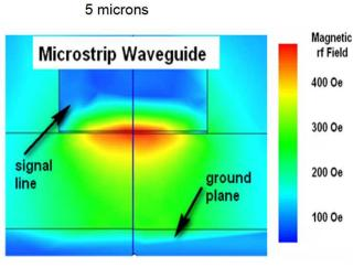
Ultrasmall waveguide geometries can produce huge oscillating microwave fields up to about 500 Oe. This is in contrast to typical cavity-based ferromagnetic resonance measurements where the oscillating magnetic field has an amplitude of about 0.1 Oe, Using these large fields, we explore nonlinear ferromagnetic dynamics in Permalloy and Fe.
